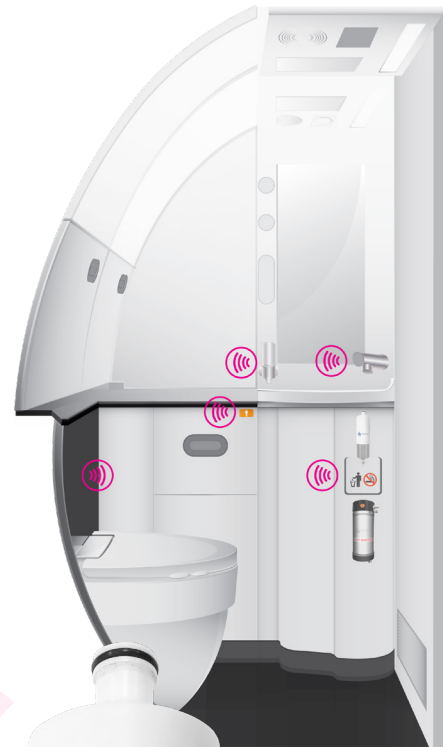
The Healthy Lav by International Water-Guard includes touchless faucet, touchless flush, the ‘HE’ (high efficiency) lavatory water heater and the UVLI LED water disinfection unit
