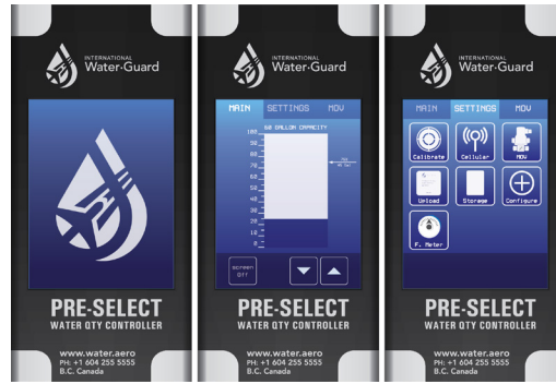
The Pre-Select Controller is an interactive Touch Screen in the aft galley's Flight Attendant Panel of the 737-8 and 737 NG that allows the Airline to pre-set the infill water quantity target in the Potable Water Tank.
