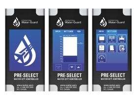
The Pre-Select Controller is an interactive Touch Screen in the aft galleys Flight Attendant Panel of the 737 NG that allows the Airline to pre-set the infill water quantity target in the Potable Water Tank.
