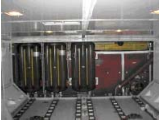
Airbus A310: original three pressurized water tanks in position in the aircraft cargo hold.
